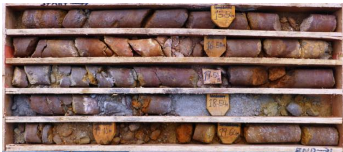
Figure 10 | Drill core typical of Composite #8; friable mineralisation over “oxide” itabirite (Zaway, ZDD001, 14.90 – 20.10 m)
