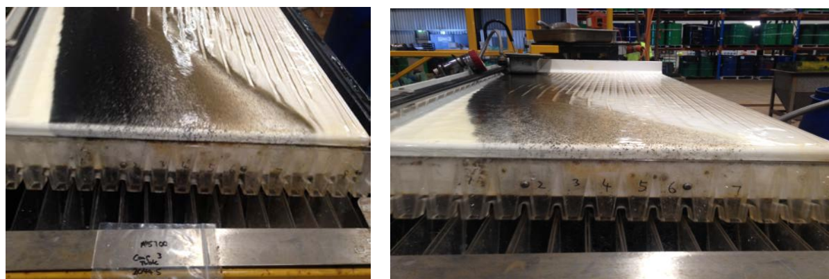
Figure 3 | Example of wet tabling conducted at ALS Perth on Composite 3 and 9
