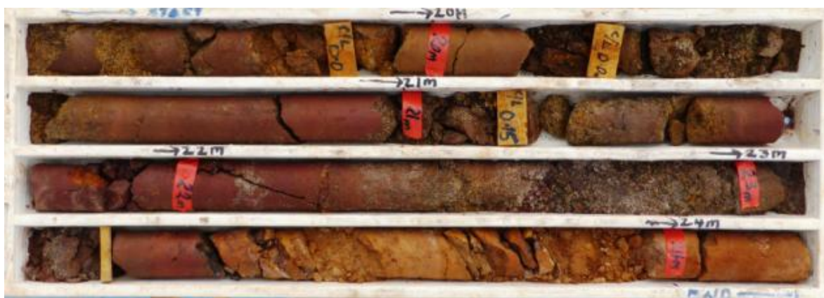
Figure 9 | Drill core typical of Composite #2; friable mineralisation over “silicate” itabirite (Gofolo, GMDD003, 19.50 – 24.16 m)
