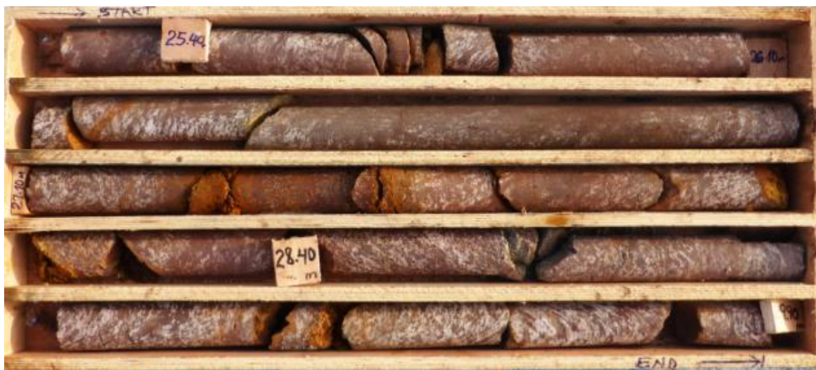
Figure 8 | Drill core typical of Composites #3 and #9; friable transitional mineralisation over “oxide” itabirite (Zaway, ZDD003, 25.25 – 29.90 m)
