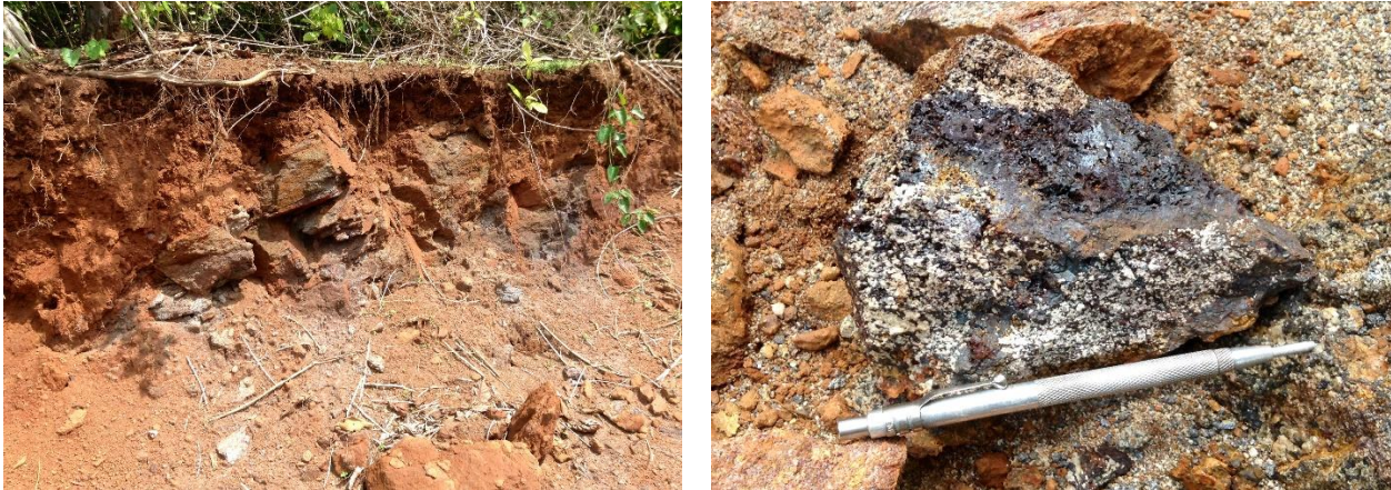
Figure 11 | Friable itabirite mineralisation in drill pad cuttings (left) and hand specimen (right) at Zaway North-West.
